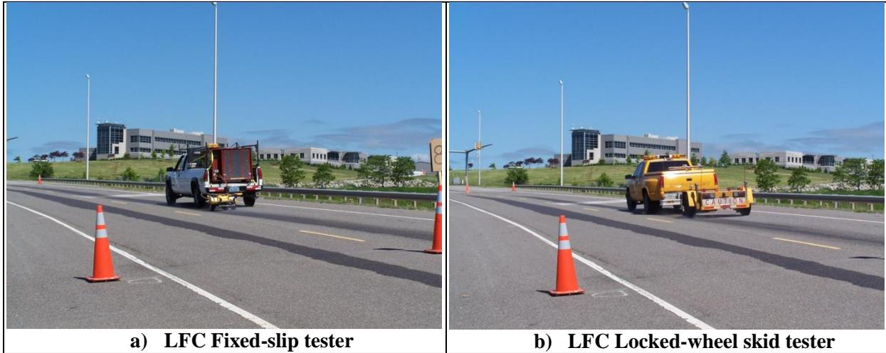
**Figure 7 Longitudinal Force Coefficient (LFC) Friction Testers**
