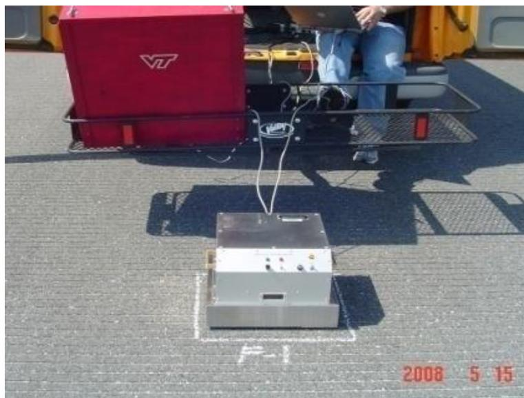
**Figure 8 Circular Track Meter (CTMeter)**
