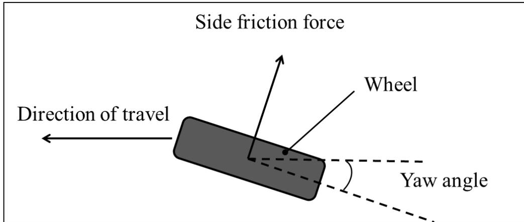
**Figure 6 Force-body diagram for a wheel traveling around a curve with constant speed (after Hall, 2009)**
