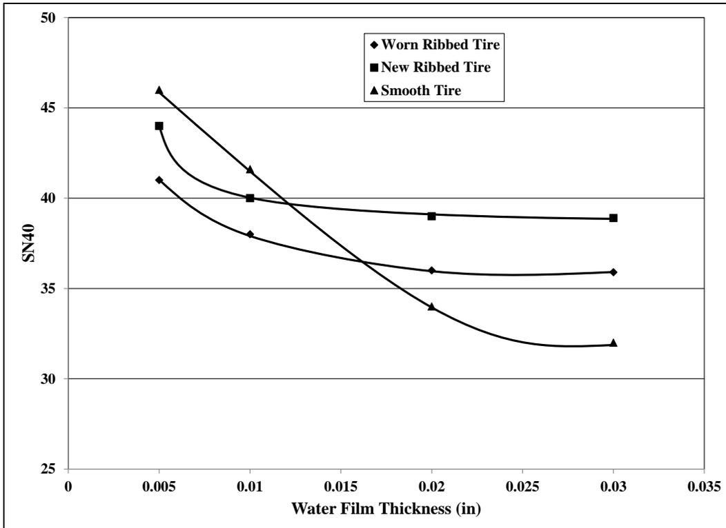
**Figure 9 Effect of water film thickness on skid measurements (after Henry, 2000).**
