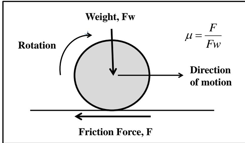
Figure 1 Force body diagram for rotating wheel
